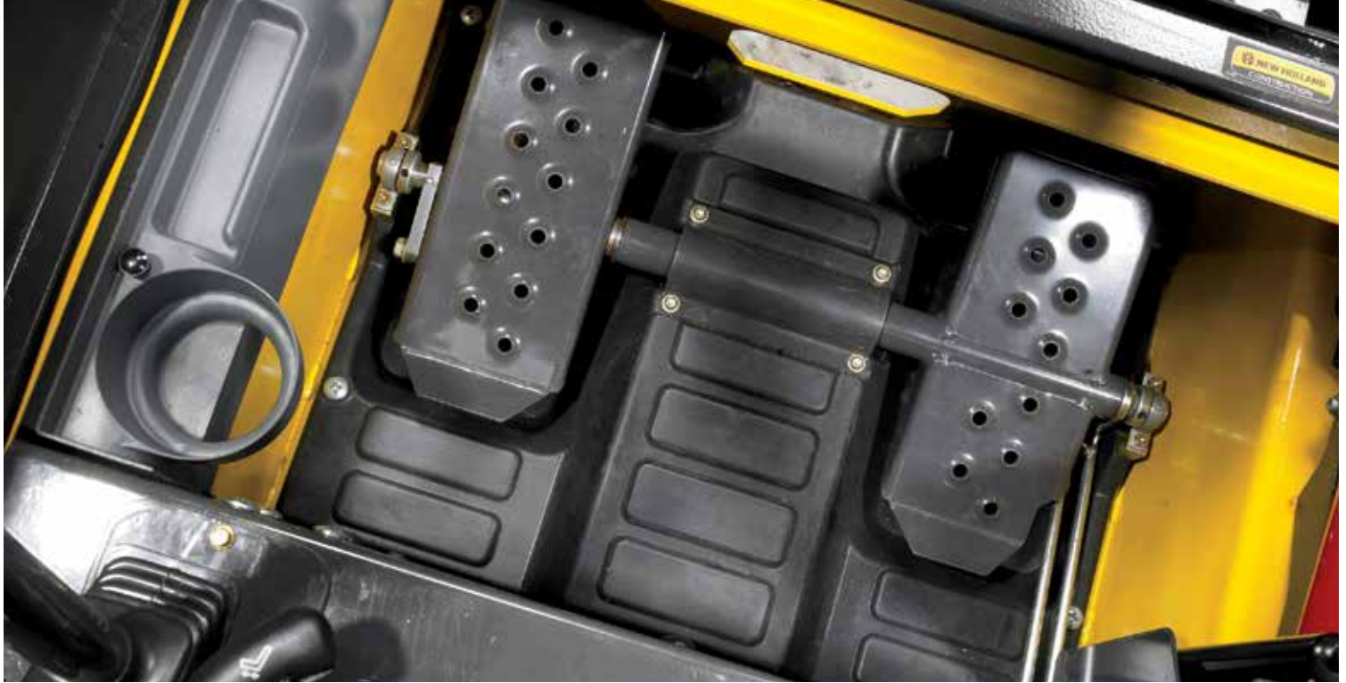
The step floor is flat for easy entry/exit and more foot and leg room.
